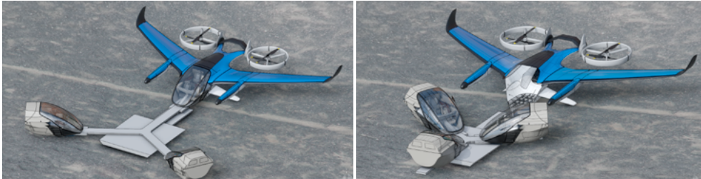
Figure 7: Cabin modularization concept for an eVTOL
