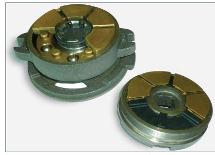
optimize the design to use a fixed box and shoes mounted on rubber. This simplification improved performance because it reverses the deformation elasticity skid to increase and retain the interposed lubricant film and permits the rubber of the shoe to oscillate in all directions."
